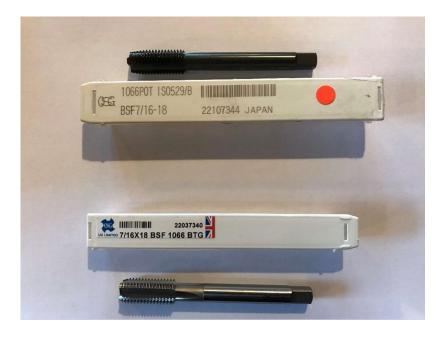
The Lower Tap (OSG 22037340) is a plug Tap for Finishing the Thread to the Bottom of the Hole.
